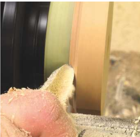
▲ Pic.13 Mount the piece for the base onto the screw, which he has shortened with a packing piece. With the gouge carefully turn a concave shape on the bottom rim
